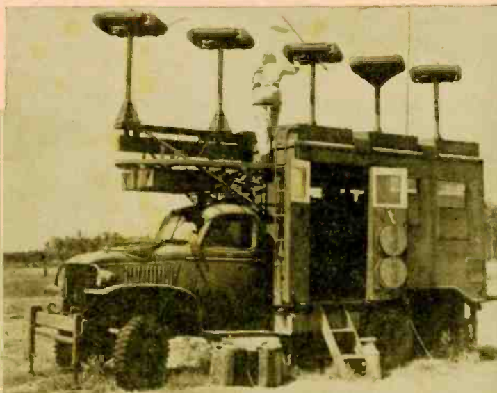
Above—Localizer transmitting unit is stationed 1000 feet from upwind end of runway and operates vertical cross-pointer needle.
